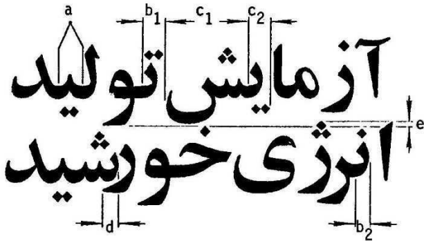
Fig. 2. Difficulties in the automatic recognition of printed Farsi texts: (a) Connectivity of symbols, (b) Similarity of symbols, (c) Variable-width symbols, (d) Overlapping subwords, and (e) Overlapping lines of texts.
